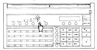
Select the required resolution. Press the resolution key repeatedly until the lamp next to the required setting is lit.
